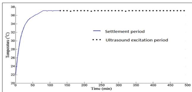
**Figure 5:** Temperature monitoring on the substrate where cells lie during ultrasound exposure. During the 6 h ultrasound excitation period (dotted line), no meaningful increase in temperature occurs, showing that heating is not the cause of the bioeffects observed on cells
