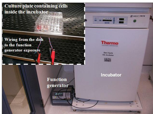
**Figure 1:** Experimental arrangement for the ultrasound exposure of cancer cells under incubation
