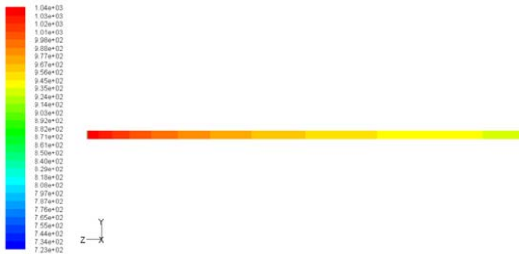
Fig. 14. The effect of a 450 °C temperature at the reactor inlet on the temperature contour inside it
