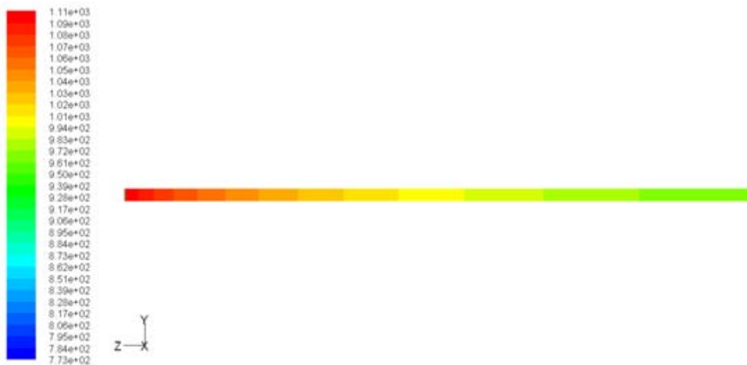
Fig. 15. The effect of a 500 °C temperature at the reactor inlet on the temperature contour inside it
