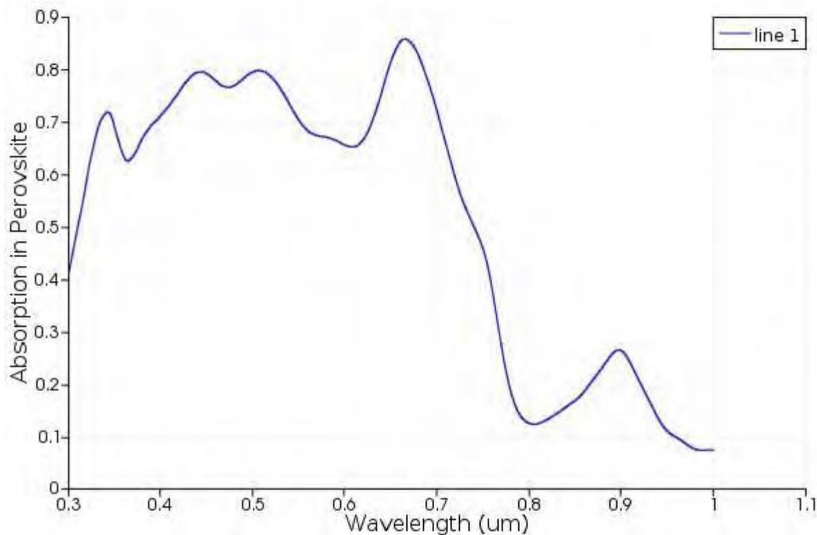
Figure 3. Perovskite solar cell absorption size diagram
